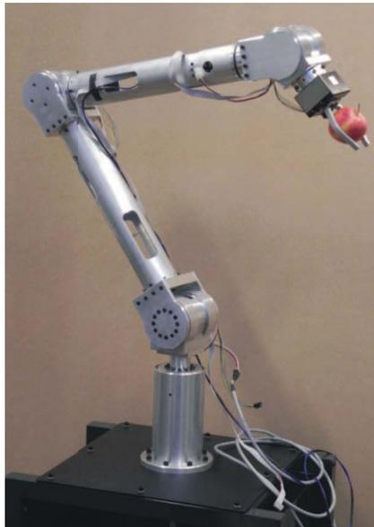
**Figure 4.15:** Prototype of the 5-dof robotic arm.
