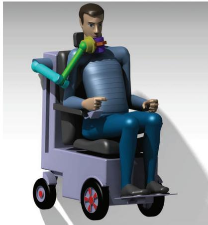
**Figure 1.1:** A lightweight anthropomorphic robotic arm mounted on an electric wheelchair.
